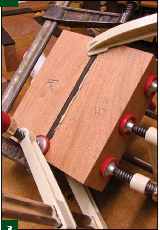
**3** **Add the accents.** Dennis chose ebony for the accents, but any complementing dark wood would work. Sand the glue surfaces of the box blank and accent blank with 80-grit sandpaper wrapped around a flat block. Remove the sanding dust with compressed air and a rag. Apply a bead of glue on both surfaces and use a paint roller to spread the glue. Clamp the pieces tightly and let the glue dry overnight.
