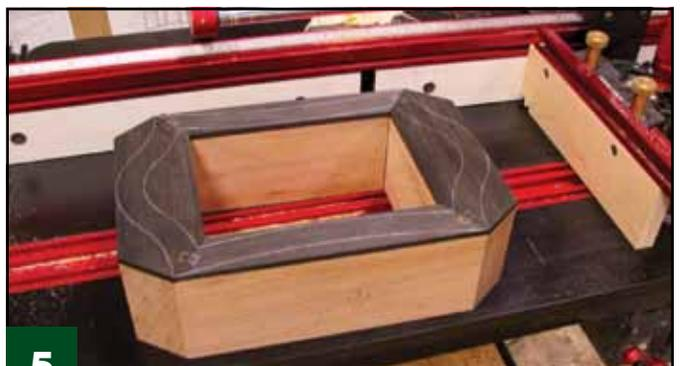
**5** **Prepare to cut the dovetails.** Use the templates to draw the shape of the box on the dry-assembled blanks. Make sure you include the dovetail lines. Cut 37° angles opposite to the 53° angles on the sides so you have a square edge to hold against the router table fence. This allows you to cut accurate dovetail slots with a router table.
