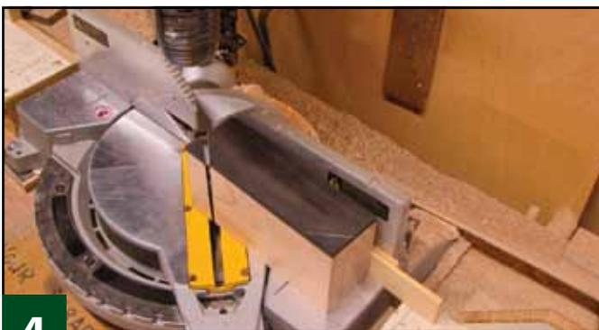
**4** **Cut the miters.** Draw the angles onto the blanks with a white pencil. Draw a 53° angle on the ends of the box sides and a 37° angle on the ends of the front and back pieces to produce the 90° angle required for the joint. Keep the side you cut off of the laminated side pieces toward the center of the box so the glue joint does not show when assembled. Cut the angles on a miter saw. You may need to add shims between the blank and the mitre saw fence to cut the 53° angles.
