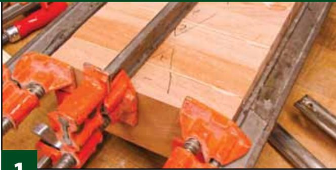
**1** **Laminate the blanks for the sides.** Sand the two surfaces to be glued together with a flat sanding block and remove the sanding dust with compressed air and a soft rag. Mark the top edges and apply Titebond III wood glue to the surfaces to be glued together. Spread the glue with a good-quality paint roller and clamp the pieces together tightly overnight. Use a jointer to square up the laminated sides.
