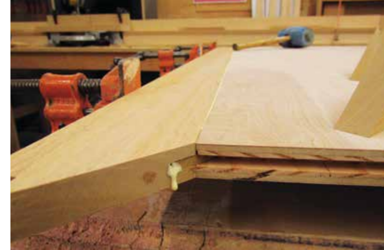
Brush yellow glue onto both ploughs and splines for each edge
