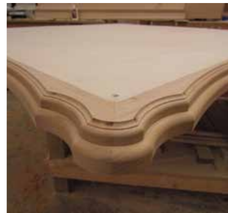
This photo shows the two stacked tops, which are stacked upside down
