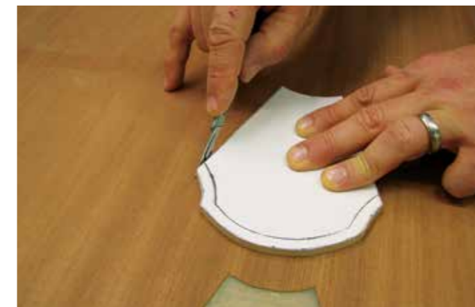
Cutting out the middle corner veneer (2)
