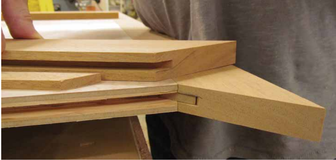
Parts for the stacked top showing top, edge and spline
