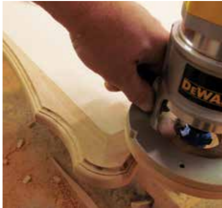
Rout in the profile edge into the bottom edge of the lower stacked top
