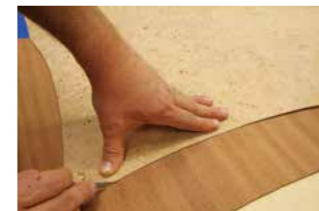
Use the centre maple burl veneer as a guide to cut out the four large borders
