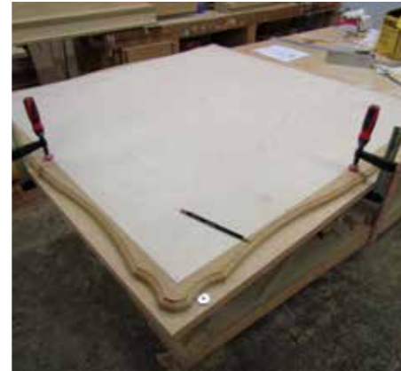
Clamp the two tops together while drawing in the offset lines to ensure accuracy that the tops won't move
