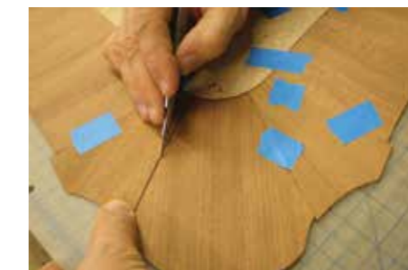
Cut the veneers flush to each other
