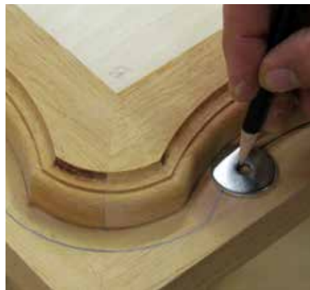
Use a washer and pencil to draw in the offset into the upper stacked top
