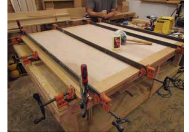
Clamping the mahogany edges to the top
