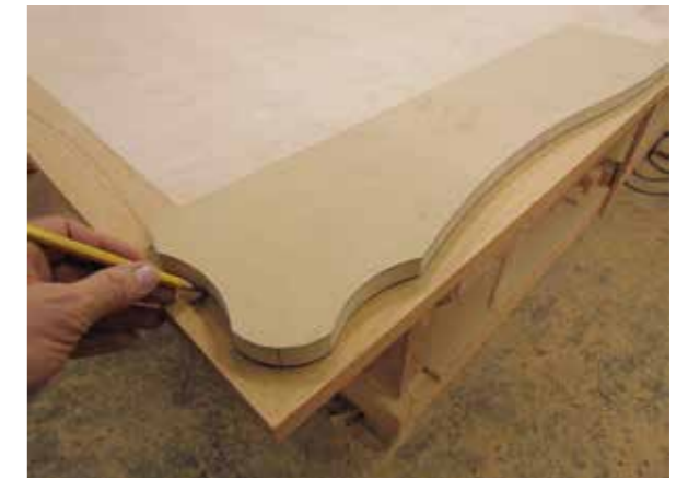
Set template 'A' on the front edges of the stacked top and trace
