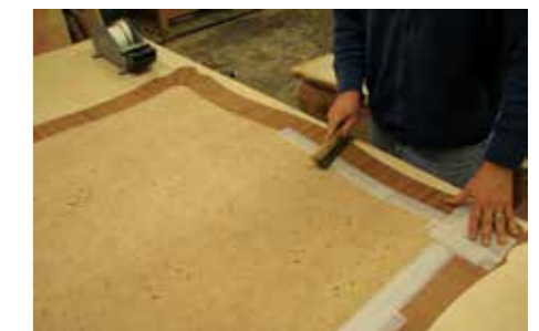
Rub down the water gum tape using a fine bristle brush
