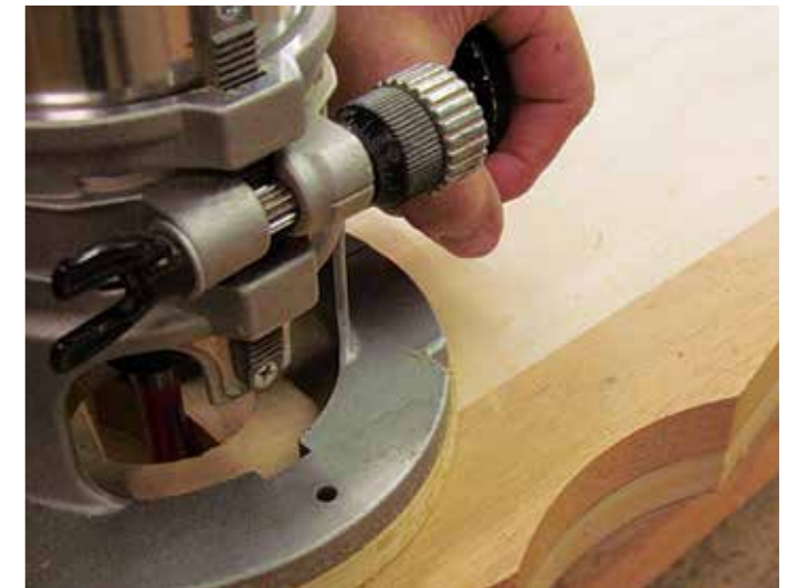
Rout the mahogany flush to the template
