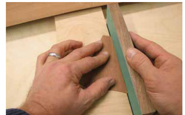
Use a sanding block to adjust the angle if needed and straighten the veneer edge
